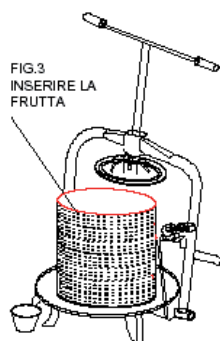
Fig. 3 - Pour the minced fruit in the cage after placing a container under the outlet spout.
